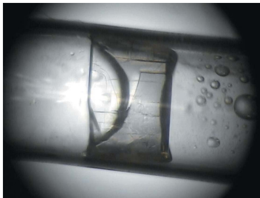
Figure 3 Photograph of the crambin crystal used for neutron diffraction data collection, measuring 3 \times 2 \times 0.7 mm ( 4.2 mm 3 ).
